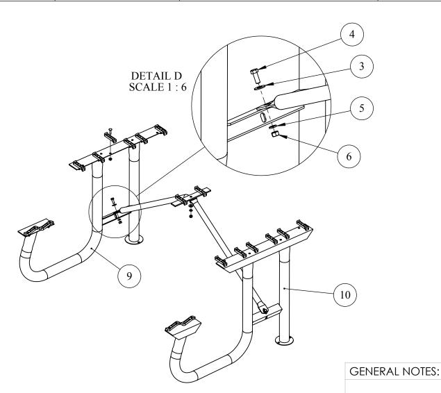
Start by Laying One of the 8' Planks Upside Down on a Flat Surface. Place a Plank Clip Under the Angle Iron Mounting Cleat of the Leg Assembly As Shown Below. Finger Tighten (2) 5/16"- 18 Flanged Nuts on Each End on the Plank.
