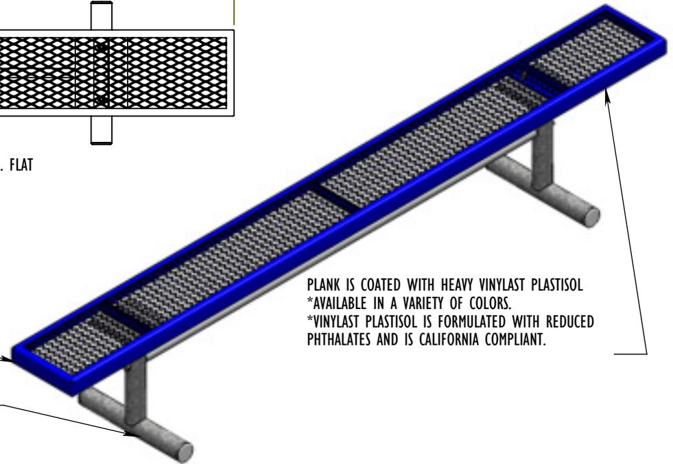
PLANK IS COATED WITH HEAVY VINYLAST PLASTISOL
