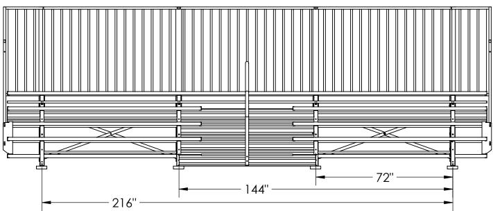
Frames are fabricated from 2" x 2" x 3/16" 6061-T6 aluminum angles. X braces are fabricated from 3/8" x 1-1/2"6061-T6 aluminum flat bars.
