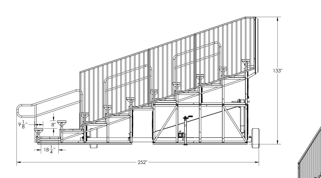
2"X 10" EXTRUDED ALUMINUM SEAT— PLANKS WITH ANODIZES FINISH
