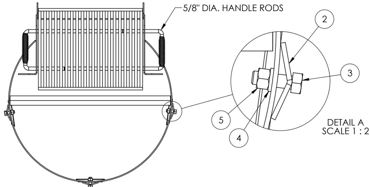
3/16" STEEL GRATE SUPPORT AND HEAT SHIELD PANELS THIS ALLOWS (4) LEVELS OF GRATE ADJUSTMENTS
