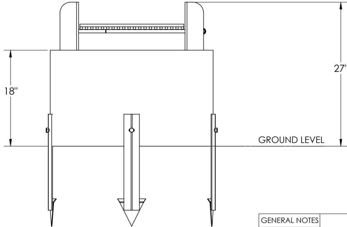
1. Before the assembly mark line on the ground the out side the grill for anchor spade placement and at as same time mark the center line where is bolts mount to grill.
