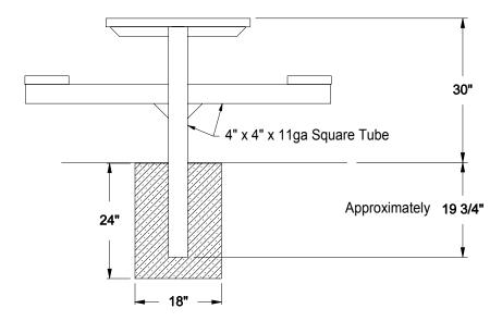
1. Soil conditions will determine the actual size of concrete footing. We recommend an 18" square hole. Set the the frames in and secure them in place. Be sure they are all level and parallel with a string line or other method. Fill the holes with concrete.
