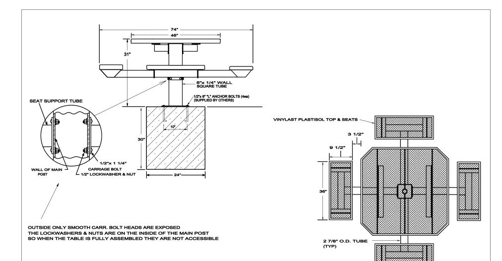
THE SIZE OF THE CONCRETE BASE IS ONLY A SUGGESTION YOUR LOCAL SOIL CONDITIONS SHOULD DETERMINE WHAT IS NECESSARY TO ENSURE A STABLE MOUNTING
