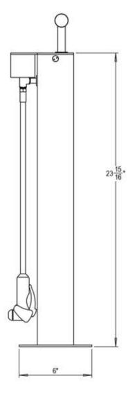
ALUMINUM HANDLE-STAINLESS STEEL COVER AND PUMP SHAFT LIQUID FILLED AIR GAUGE STEEL HOUSING AND FLANGE PRESTA AND SHRADER VALVE HEAD
